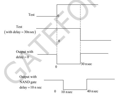
So we can clearly say that initial output change from high to low, then it changes from low to high and then finally at steady state output is 1.
